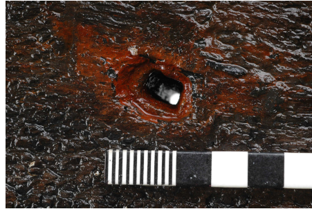
Figure 3.4 The imprint of the head of the wrought iron nails. Photo: L. de Jong.
